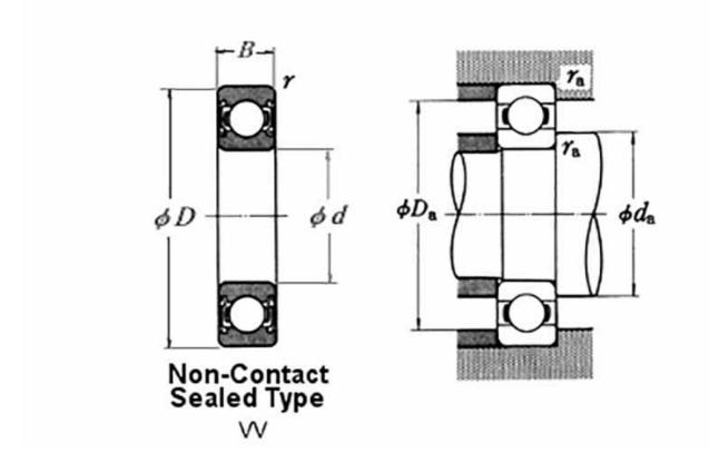
High quality Deep groove ball bearing with non-contact rubber seals from the world leader NSK, the worlds largest ball bearing manufacturer offering unparalelled quality. The unique & patented NSK VV rubber seal features market leading technology, keeping contaminants out of the bearing while retaining the high class lubricant inside. The non contact design ensures low torque and therefore very low power loss
